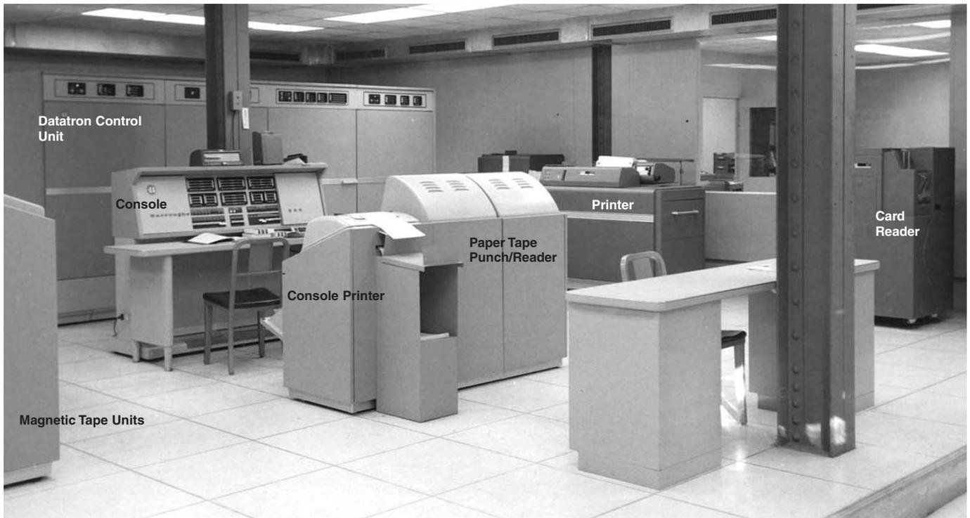
Figure 5. Burroughs 220 computing system in Rand Hall
